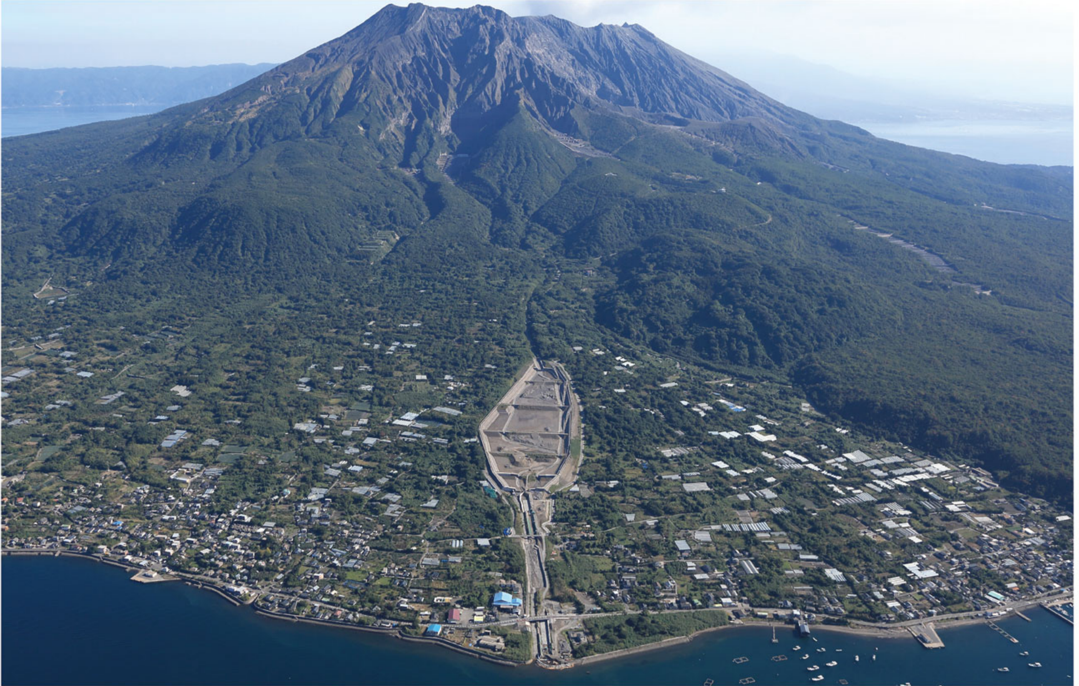
Sand retarding area for volcanic debris at Sakurajima in Japan, designed by Nippon Koei (Photo: Osumi River and National Highway Office, Ministry of Land, Infrastructure, Transport and Tourism)
