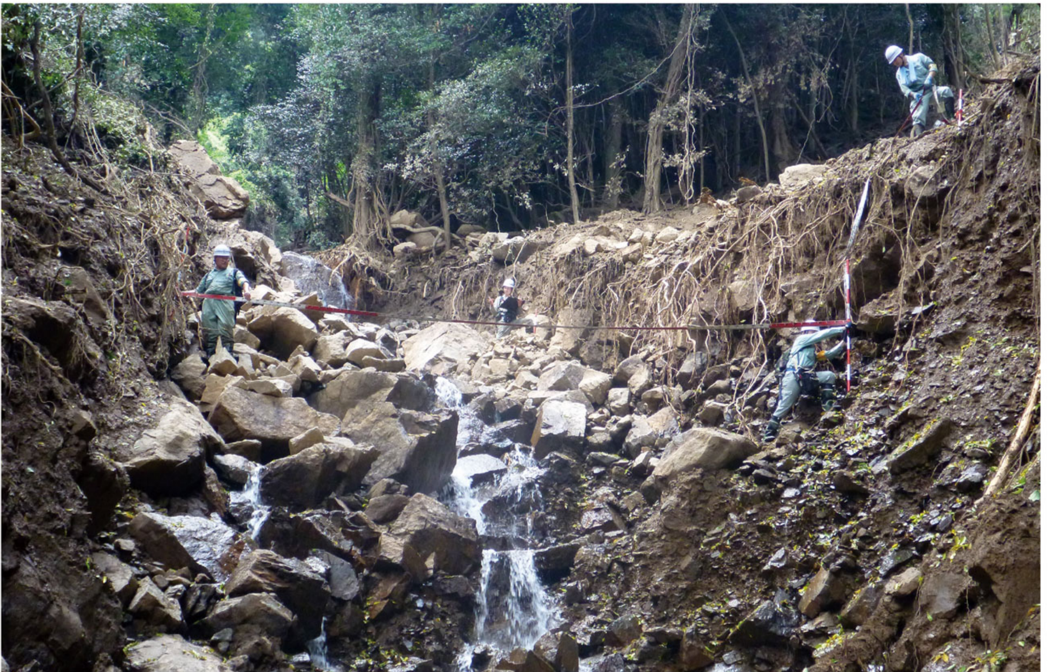
Survey of torrents with debris flow hazard for developing debris flow countermeasure plan
