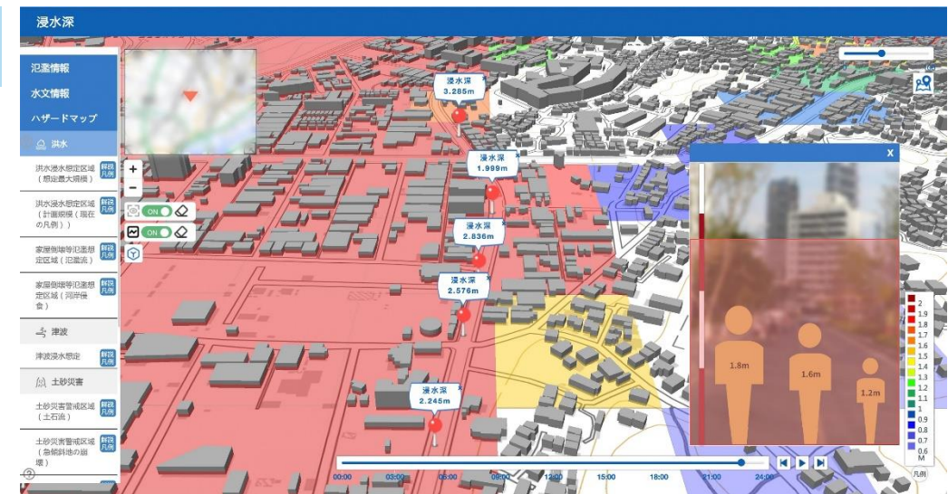
Screen image*3 (Real-time flooding analysis results and flooding sensor information)
