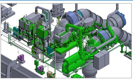
The method is used to visualize the final shape of a 3D model of machine equipment (gray) and point cloud data (green)
