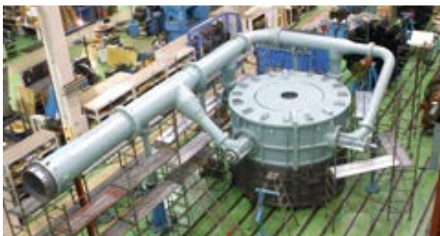
Vertical Pelton turbine being assembled at a factory
