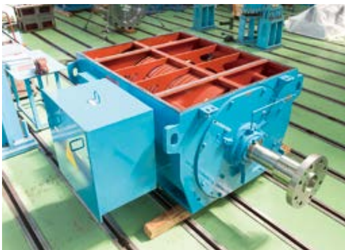
Horizontal induction generator
